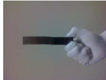
Figure #5 - Gage Blocks Wrung Together
